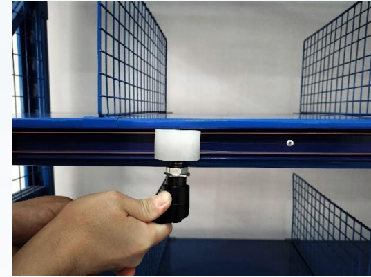
3、 Press the copper wire into the slot with press wheel
