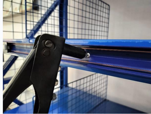
2、 Drive the rivet into the hole with a rivet gun
